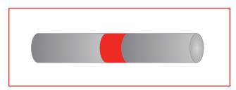
**CYLINDRICAL JOINT:** A cylindrical joint uses a butt joint to join two cylindrical objects.
