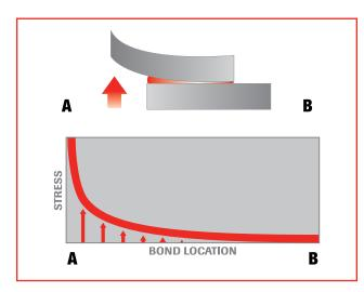
**PEEL STRESS:** A peel stress occurs when a flexible substrate is being lifted or peeled from the other substrate. *NOTE: The stress is concentrated at one end.*
