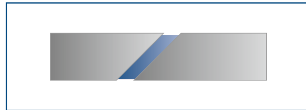
SCARF JOINT: A scarf joint is an angular butt joint. Cutting the joint at an angle increases the surface area.
